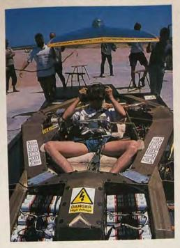
Power came from the sun via an 80 kg removable solar array being fitted over codriver Viv Baddeley (above) before a shift behind the wheel on the Nullarbor Plain. Ahead stretched three hours of cramped, humid driving reclined in the cockpit 70 cm above the ground.
